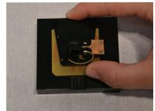
6. Using the tips of very sharp tweezers, pick up the new probe and, while pressing down on the probe holder, gently slide the probe into place. Take care not to touch the
