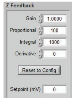
4. *Derivative*: Scale factor for the derivative term in the PID feedback controller.
