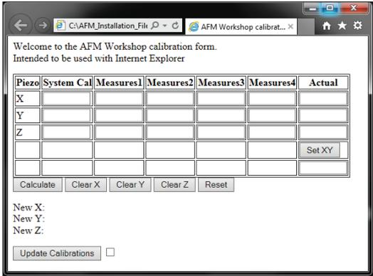
3. Insert the current calibration values, located on the System tab, under System Cal in the calibration software.
