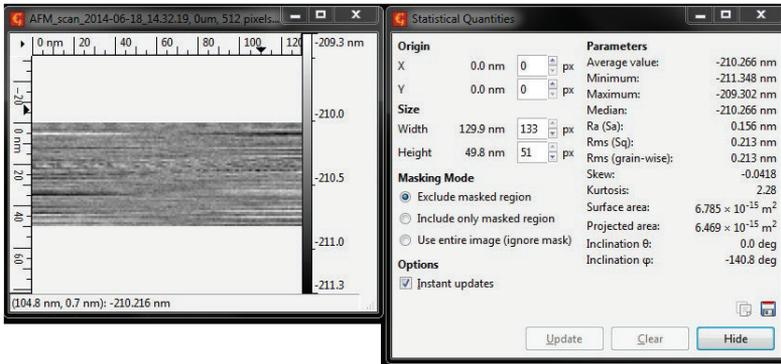
Noise can be reduced by lowering the Z HV Gain in the System tab. When the Z gain is lowered, a new tip approach must be initiated because the Z ceramic's dynamic range has been reduced.
