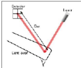
The deflection of the cantilever can be converted to Force using Hook's law:
