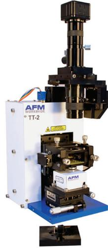
TT-2 AFM stage combined with the video microscope
