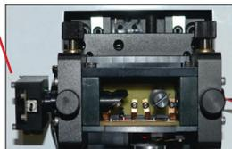
15. Move the L-R signal to zero by adjusting the detector translation thumb screws.
