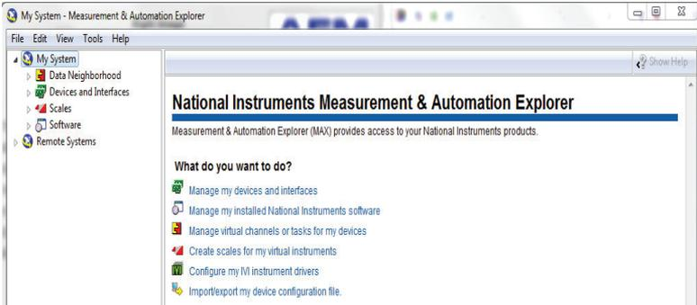
1. Expand Devices and Interfaces under My System on the left scroll tab.
