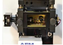
3. Place the probe holder on the probe exchange tool with the spring facing up.
