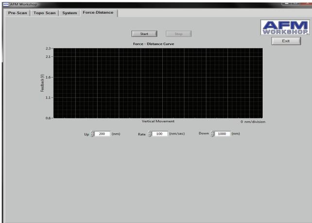
The AFM must be in feedback in non-vibrating mode before a F/D curve is measured. There are three important parameters that must be set before the F/D curve is measured. They are:
